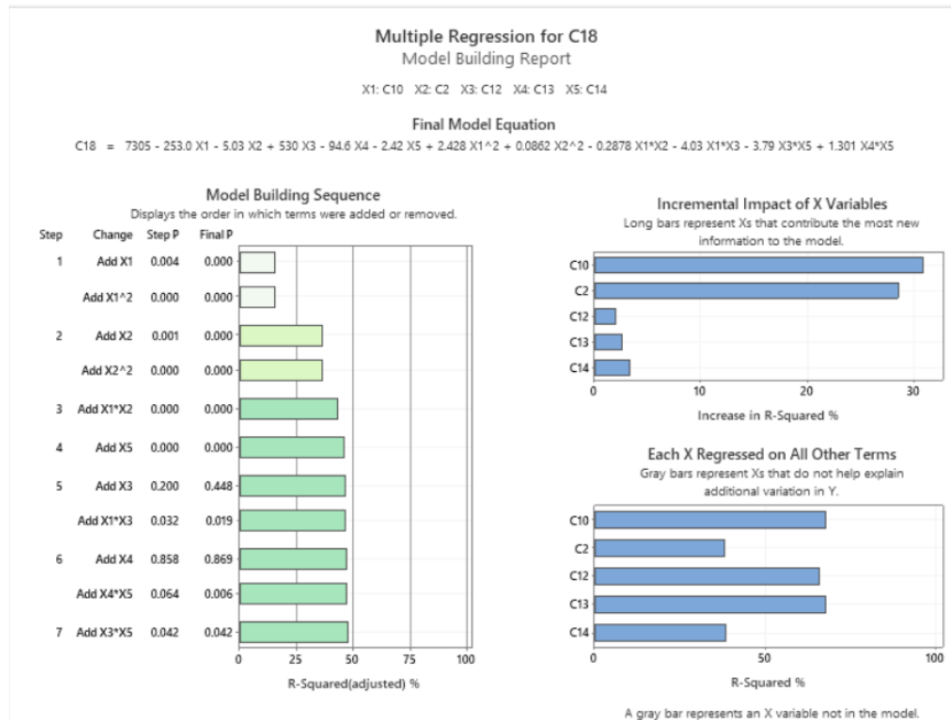
Figure 9. How the equation uses each term in the polynomial to reduce the error and improve the r-squared
